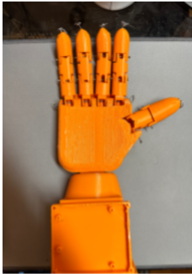
Figure 17: 3D printed prototype 1 (Made by T. Tran in Solidworks, 2023).
