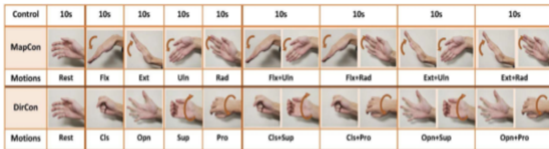
Figure 4: MapCon and DirCon. Common myoelectric movements with MapCon and DirCon control (Zhu et al., 2022).
