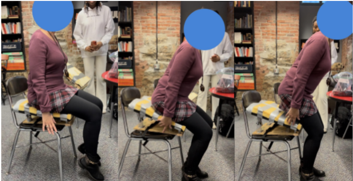
Figure 11: Client testing the final prototype. Note: the cover for the cushion is not shown here, but it serves no mechanical purpose.
