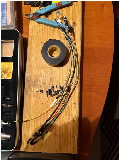
Soldered wires and transistors onto vibration motors
